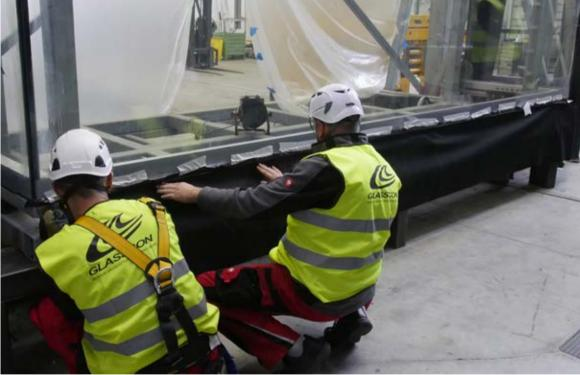
The VMU was dismantled by GLASSCON's team from the site and re-installed at an accredited European testing institute (NANDO certified members) for testing. The same installation team was used at all related works to guarantee the highest quality of installation work at the project final facade.
