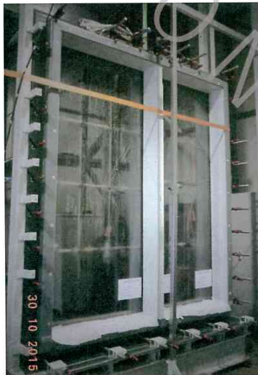
Photo 2. Tested sample undergoing watertightness test
